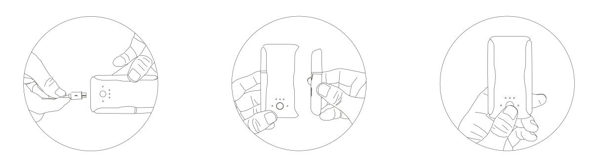
2. When you are ready to charge the Charging unit, align the charging cable with the USB charging port and the other end for the power connection.
