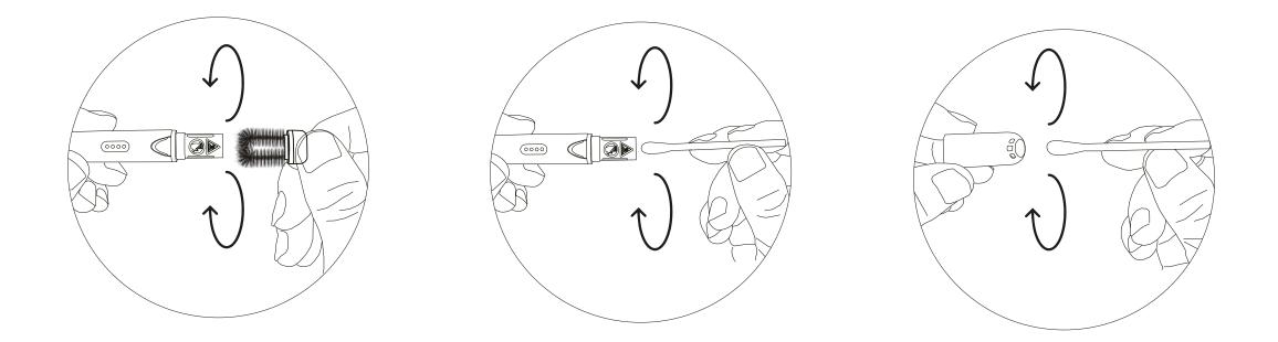
1. When cleaning the ISMOD holder, pull out the protective top cover of the ISMOD holder, insert the cleaning brush according to the following picture, turn it several times, then remove the residue on the cleaning brush, and afterwards, use the cleaning sticks and finish with the cleaning plate.
