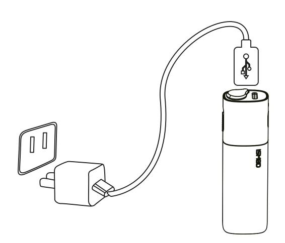
Connect the USB cable to the charging adapter.
