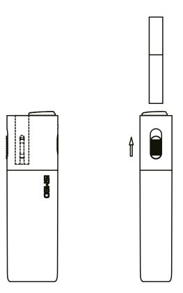
(2) Remove the non-combustible tobacco cartridge and twist the protective cap
